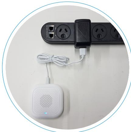
Connect the Gateway to a USB Power Adapter using a Micro USB Cable.
